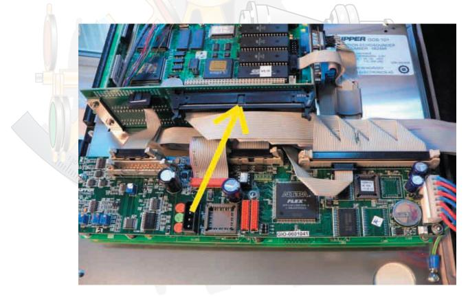
WHAT TO DO: When inserting the buscable into the motherboard, ALLWAYS insert and take out 2 or 3 times to ensure best possible contact in plug.
